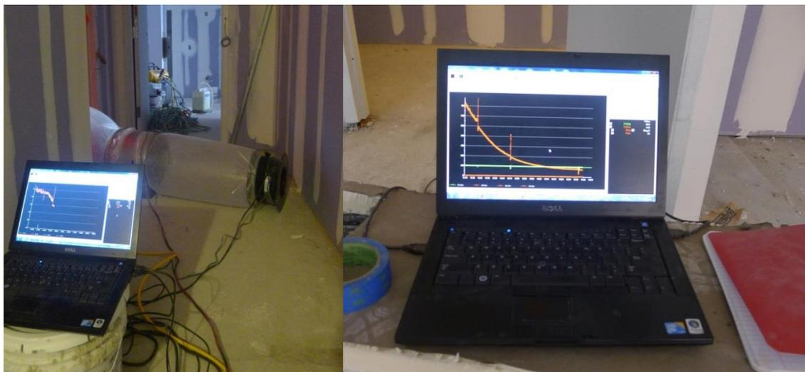
Figure 15 displays the sealing profiles for four apartments and shows that the process was capable of sealing at least 80% of the air leaks in less than two hours. The plateau in sealing rate occurs when all smaller leaks are sealed (<0.5 inch in the smallest dimension) and only large leaks that cannot be sealed by the aerosol process remain. This plateau occurs at different points depending on the building's initial bulk-sealing level.
