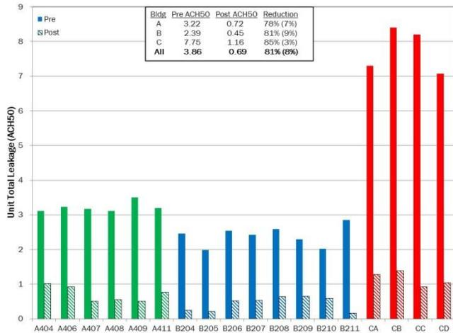
As shown in Figure 6, results were equally impressive for existing buildings, sealing an average of 68% of the unit leakage. The tightness achieved was less consistent for two of the tests, where only 39% of the available leakage was sealed. In one case this was due to large unforeseen leaks behind a kitchen cabinet.
