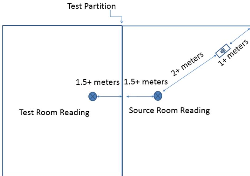
A background noise measurement is recorded prior to all sound level measurements. A handheld decibel meter is used to confirm that the sound produced by the speaker is at least 10 dB above the background noise (this is especially important in the room without the sound source). If the sound produced by one speaker is too low, a second speaker is used. A total of 4 background sound level measurements are recorded per sealed unit:
