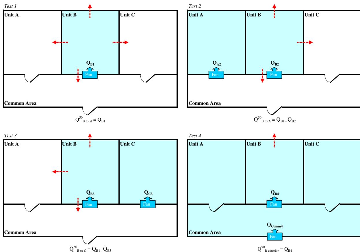
Test 1 was used to determine the unit’s total air leakage. A second fan was installed in the hallway door of unit A for the second test. The fan in unit B was adjusted to produce a 50 Pa pressure for unit B relative to outdoors and the fan in unit A was adjusted so that the pressure difference between units B and A was zero<sup>7</sup>. The difference in the air leakage for the first two
