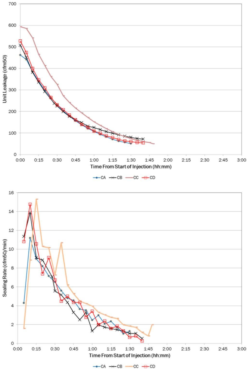
For almost all of the units the sealing rate peaked in the first 15 minutes and then steadily decreased. The pattern of leakage reduction was consistent for five of the six units in building A
