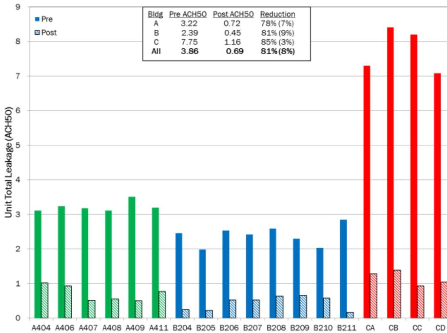
**Table 11: New construction building pre/post aerosol sealing leakage test results**
