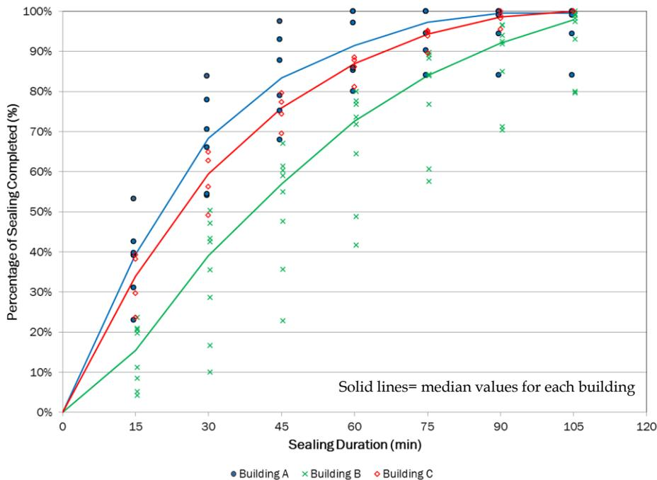
The slower sealing for some of the units in building B was caused by equipment malfunctions that were partially due to the inexperience of some of the field staff. In addition, for some of the building B units the time required for the sealant to travel from the pump to the nozzles was included in the sealing time. For the latter buildings a higher initial sealant flow rate was used
