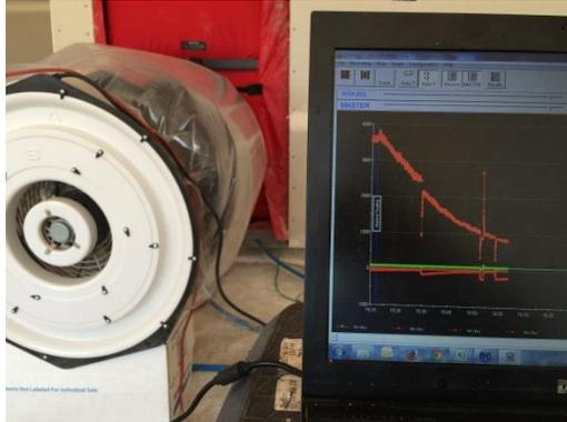
2. Monitor the calculated indoor relative humidity and/or compute the required sealant injection rate. Adjust the sealant injection rate to achieve a relative humidity of about 90%.
