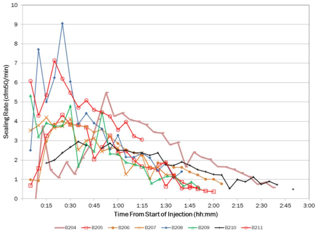
Figure 29: Variation in unit leakage (top) and sealing rate (bottom): Building C
