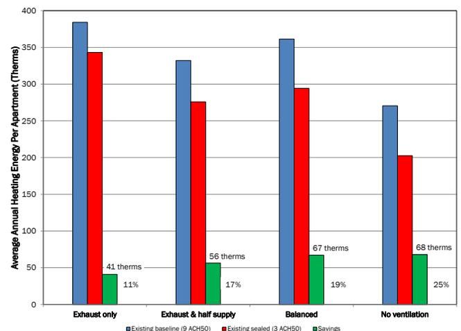
The results show an 11% to 25% reduction in heating energy use due to sealing the envelope with annual gas savings of 41 to 68 therms and cost savings from \$24 to \$39, which may not be sufficient for many building owners. However, the modeling results were based on a 68% reduction from a starting leakage of 9.5 ACH50, and the
