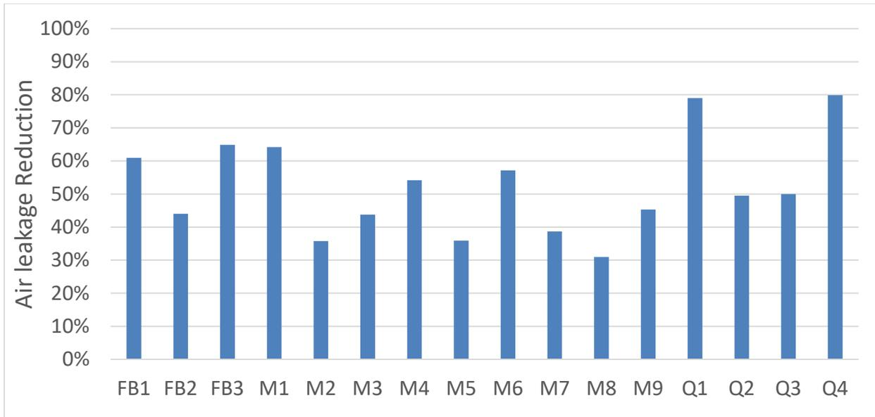
**Figure 16: Percent air leakage reduction for all demonstrations**
