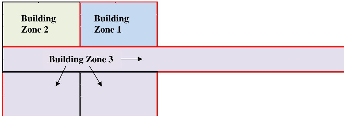
**Figure 17: Diagram of Ashurst Elementary wing sealed with red border indicating where manual sealing was performed at the roof-to-wall interface and building zone numbers corresponding to results shown in Table 2.**
