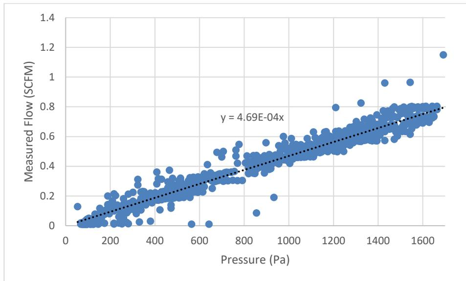
**Figure 33: Measured flow vs. pressure of test apparatus**
