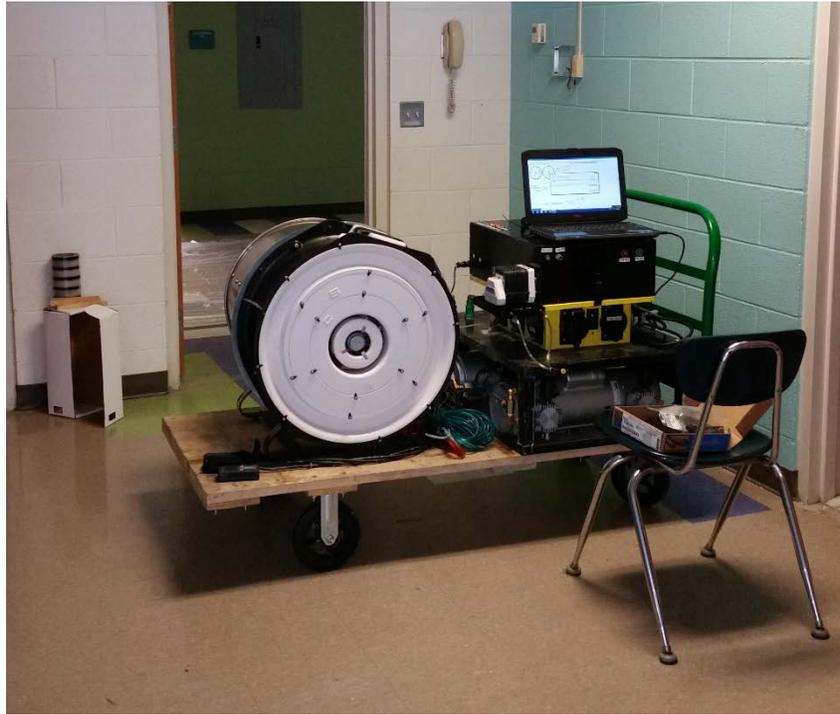
**Figure 14: Photo of aerosol sealing equipment setup**
