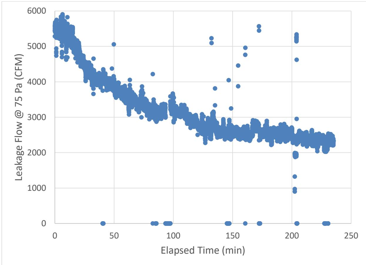
**Figure 25: Sealing profile for building M2338 at Fort Bragg Army Base**
