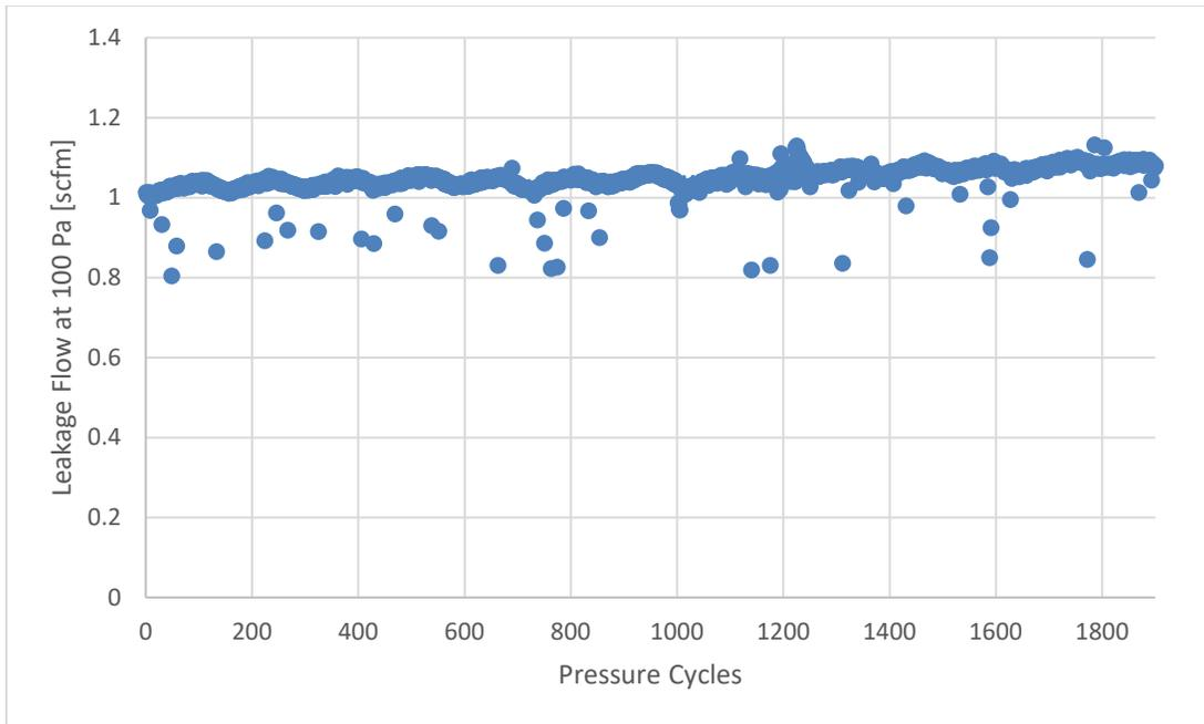
**Figure 40: Leakage rates over 1,900 cycles of 100 Pa**
