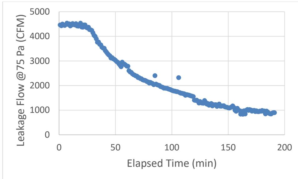
**Figure 19: Sealing profile for building 2177 at Quantico MCB**
