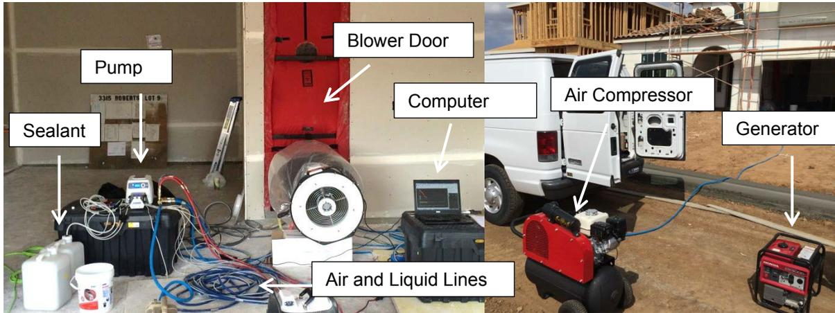
**Figure 7. Primary equipment used for aerosol sealing installation**
