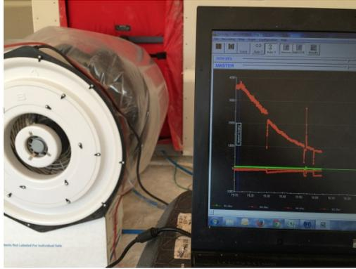
**Figure 11. Sealing underway and results being plotted in real time**
